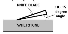
At first press fairly hard, using a circular or figure-eight motion, (or whatever suits you). Work all along the knife edge from the point to the base, changing sides every so often. Rinse or wipe off the knife and the face of the whetstone frequently to remove the small pieces of metal and stone that are ground off. Rinsing in water works well.
