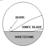
where the whetstone was used last. Check for this burr frequently during the sharpening process. Continue grinding both sides of the knife with the whetstone until you have this burr all along the edge. When this happens, all the roundness has been ground off, and there is a good edge all along the knife.
